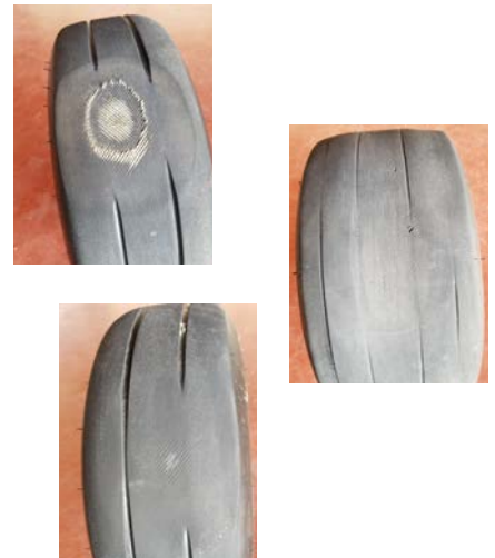
Examples of tire replacement due to abnormal wear
