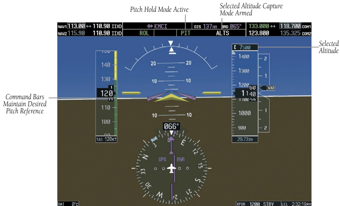
Figure 6-5 Pitch Hold Mode
