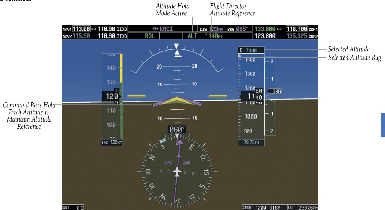
Figure 6-7 Altitude Hold Mode
